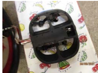
Underside of pedal secured to block with zip ties
