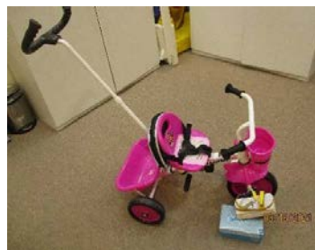
Final adaptations with non-skid seat and adapted pedals
